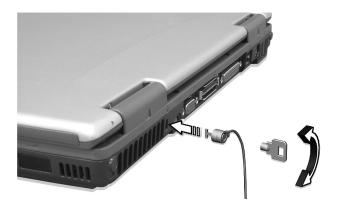
Wrap a computer security lock cable around an immovable object such as a table or locked drawer handle. Insert the lock into the notch and turn the key to secure the lock. Some keyless locks are also available.
